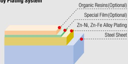
For post-treatment, various methods are offered such as oiling, phosphating, functional resin (for fuel tanks), etc. Electro-galvanized steel with these types of coating are used in the automotive industry.
