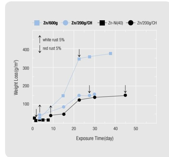
Corrosion Resistance Comparison : Pure Zn vs. Zn-Ni
