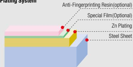
For post-treatment, various methods are offered such as no treatment, oiling, phosphating, anti-fingerprinting, black resin, etc. Electro-galvanized steels with these types of coatings are popular in the home appliance industry.
