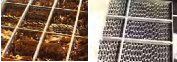
Regular steel used (serious corrosion shown) Sulfate resistant steel used (excellent corrosion resistance shown)
