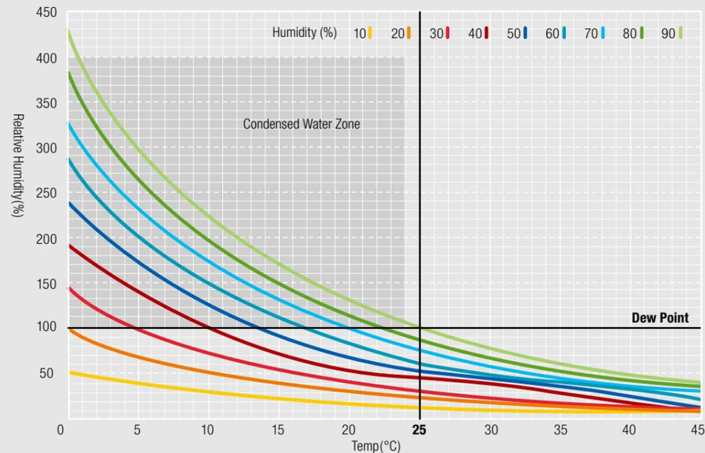
Water is condensed on the steel surface in certain temperature and humidity in store place and steel is likely to get rusty.
