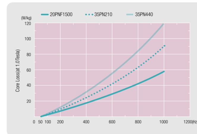
PNF-Core of 0.20mm has lower iron loss than 0.35mm product due to less eddy current loss in high frequency. 20PNF1500 has 30% improved magnetic properties(1.0T/400Hz) compared to 35PN 210.
