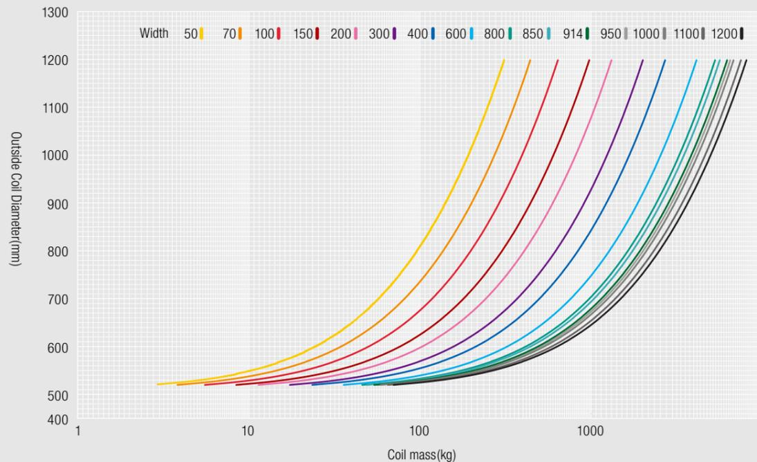
Note) Inner diameter is 20inch (508mm)
