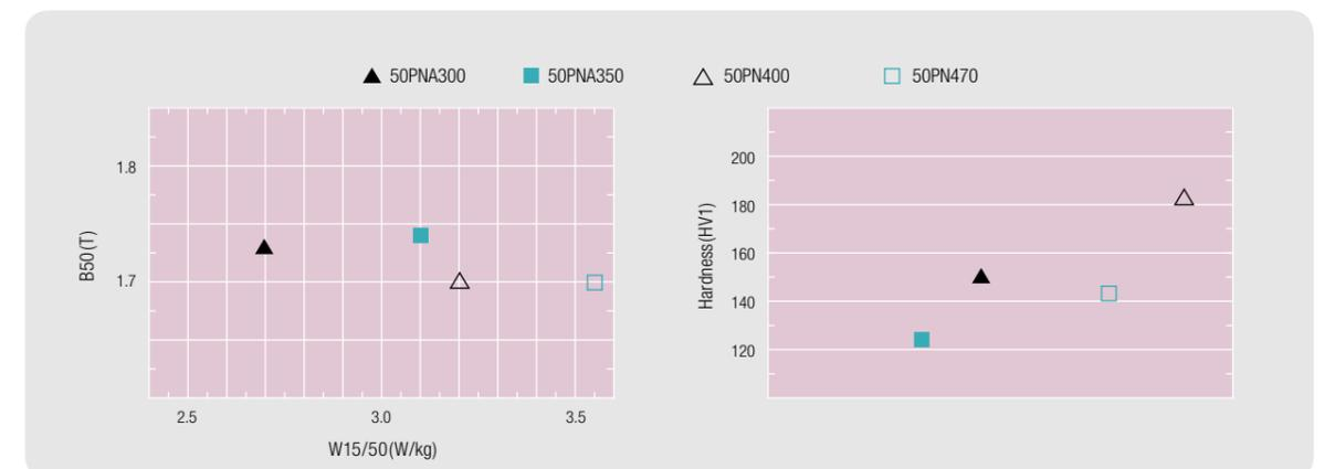
Through higher induction and lower hardness, PNA-core features higher efficiency of products and longer life of dies.
