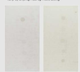
\*Checking the color difference between the surfaces after conducting a salt spray test (SST) for 48 hours following a chemical solution treatment
