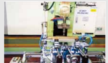
<AC Spot 溶接機: 75kVA>
