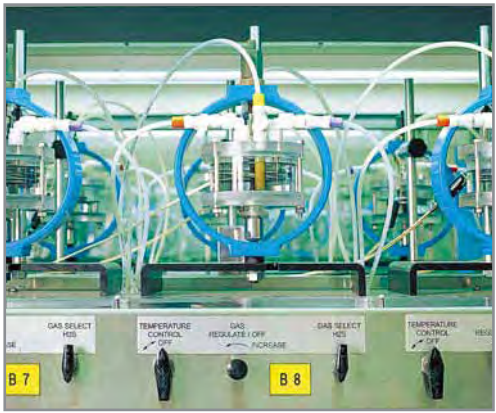
Static load method : proof ring type
